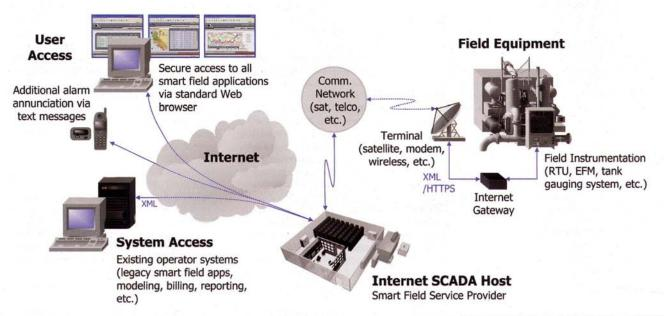
se of Internet SCADA as the basis for a cost-effective enterprise smart field system has finally moved from promise to reality. The demand for affordable monitoring and control of remote oil and gas assets is exploding, and many companies are now considering using the Internet and supervisory control and data acquisition (SCADA) to provide access to real-time data display, alarming, trending, and reporting from wells, tanks, compressors, valves and pipelines.
